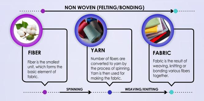
Fabric is transformed into various end products as per requirement. Textile/Apparel product development passes through the stages of planning and execution with quality control at each stages.
