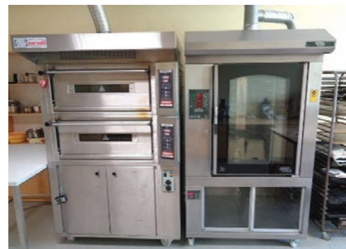
Fig. 1.47: Commercial electric oven
