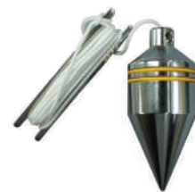
Fig. 2.4: Plumb bob and rule
