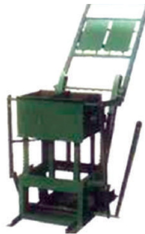
Fig. 4.5: Block casting machine
