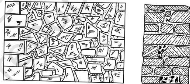
Fig. 1.11: Uncoursed random rubble masonry
