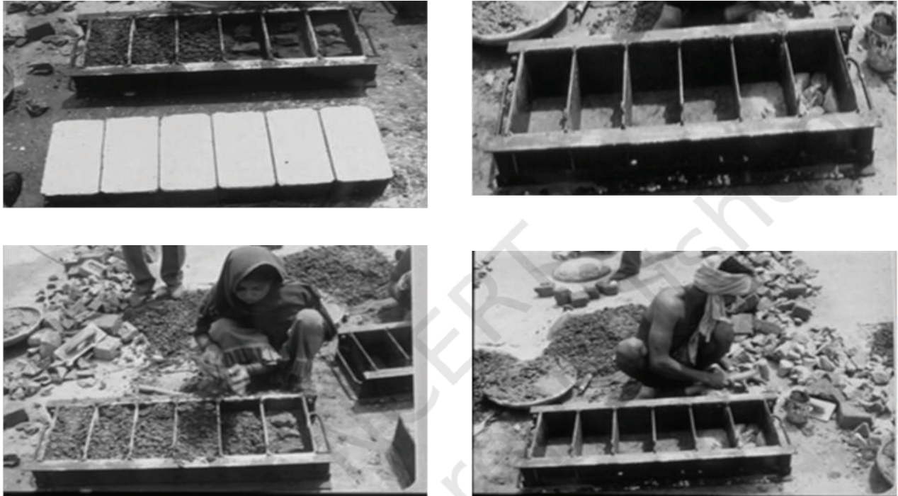
Fig. 4.8: Steps in moulding of concrete block
