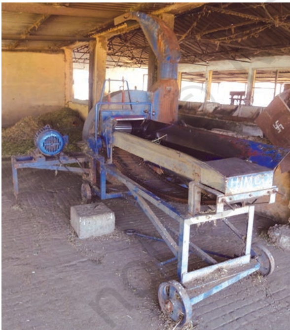
Fig. 4.8: Electrically operated chaff cutter
