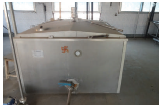
Fig. 3.5: A milk chilling tank of 1000 litre capacity
