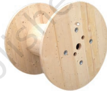
Fig. 2.21 Cable drum without cable
