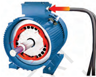
Fig. 8.23: Three-phase input supply to the squirrel cage induction motor
