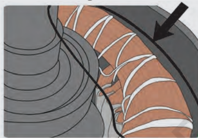
Fig. f: Winding shortened to the body
