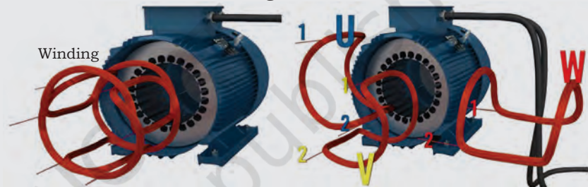
Fig. c: Three coils in the stator represented by 'U' in blue colour, 'W' in red colour, 'V' in yellow colour
