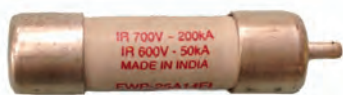
Fig. 3.16: Blown fuse, 1 - Fuse body, 2 - Striker pin ejected from the fuse, indicating that the fuse is blown
