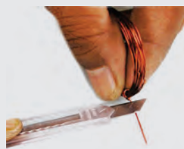
Fig. c: Remove insulation coating
