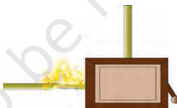
Fig. 3.2: Wire burning due to excessive current
