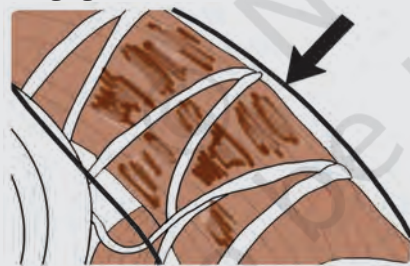
Fig. g: Ensure that the winding is not open or blown
