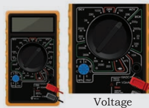
Fig. a: Setting up the multimeter in voltage measuring mode
