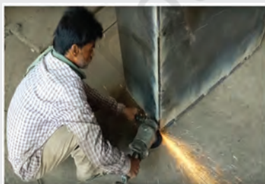
Fig. e: Making the main tank and the oil tank
