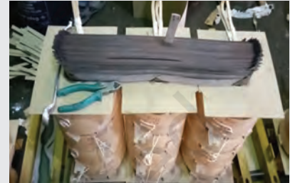
Fig. i: Insertion of I section in the core
