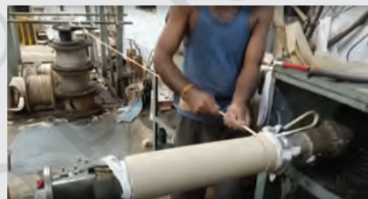
Fig. d: Making a three-phase transformer's secondary winding using a winding machine
