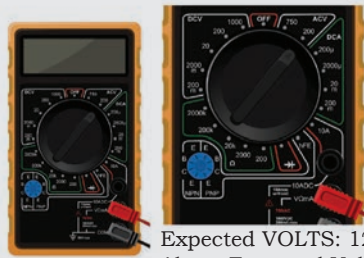
Fig. b: Setup the range of the voltmeter
