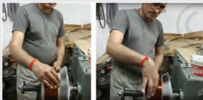
Fig. c: Making a three-phase transformer's primary winding using a winding machine in the form of a bundle
