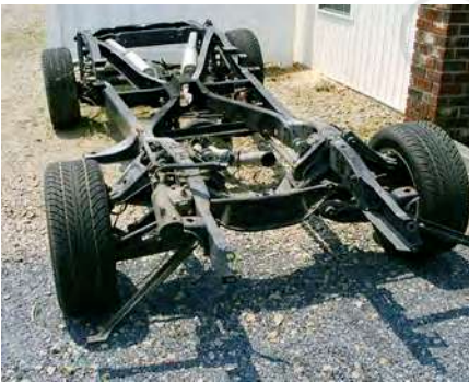
Fig. 3.1: Chassis with suspension and exhaust system
