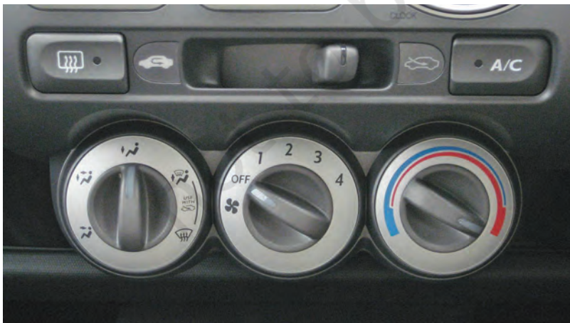
Fig. 3.37: Air conditioner in a car
