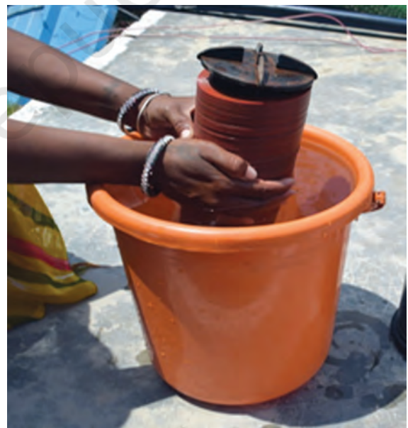
Fig. 3.8: Cleaning of disc filter
