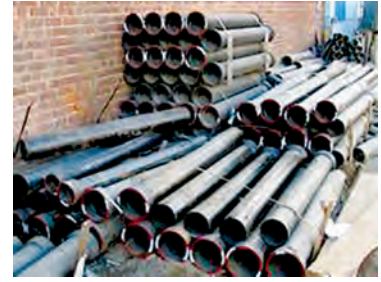
Fig. 3.4: Cast iron pipes
