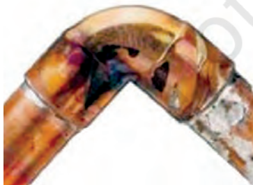
Fig. 5.24: Brazed and soldered joint
