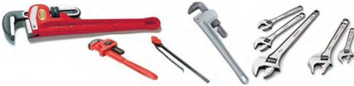
Fig. 2.4: Different type of wrenches (adjustable)
