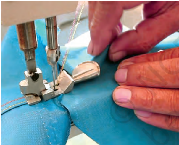
Fig. 1.6: Double chain stitch machine
